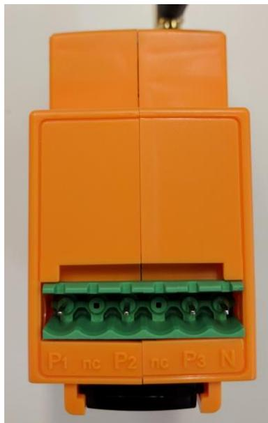
Figure 4 Voltage Supply Connection Area
