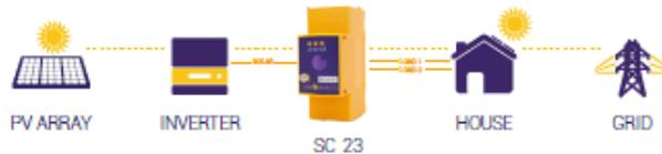
For a typical single phase application the SC-23 will monitor the solar PV plus two household circuits, e.g. hot water and total demand.
