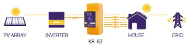
For a typical single phase application the KR-63 will monitor the solar PV plus five other circuits, e.g. whole site mains and four other household load circuits.
