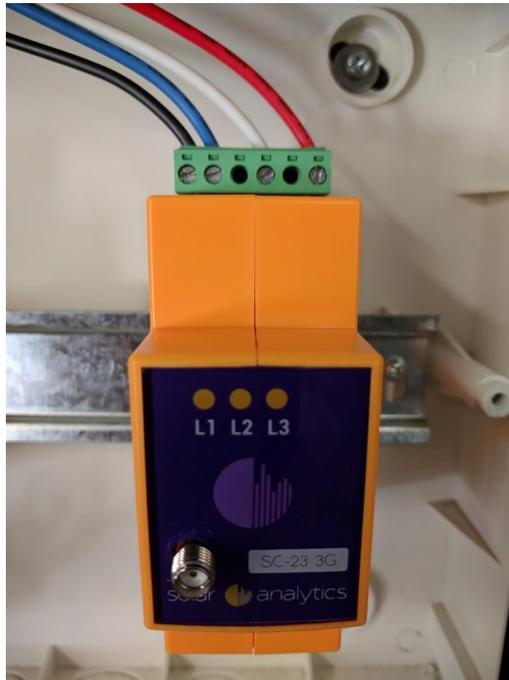
*Figure 6 SC-23 with 3 phase tail on DIN Rail*
