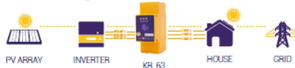
For a typical three phase application one KR-63 will monitor all three incoming phases of the solar PV system along with three remaining household load circuits.
