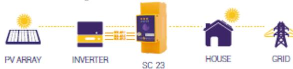
For a typical three phase application one SC-23 will monitor all three incoming phases of the solar PV system. Additional SC-23 devices can be installed to monitor additional 3 phase load circuits.
