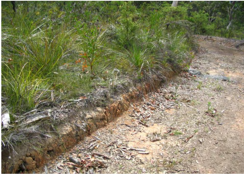
Plate 7-6: Transect 2 looking north. This shows a section of the soil profile towards the base of the moderate to steeper slopes. The upper soil unit is a recent organic layer, most likely developed from decaying organic matter, while the lower unit is the clayey B horizon common in this area. Of note is the sharp contrast between the two units, which indicate that the topsoil has moved from upslope through colluvial process truncating the in situ topsoil, which has now moved downslope.
