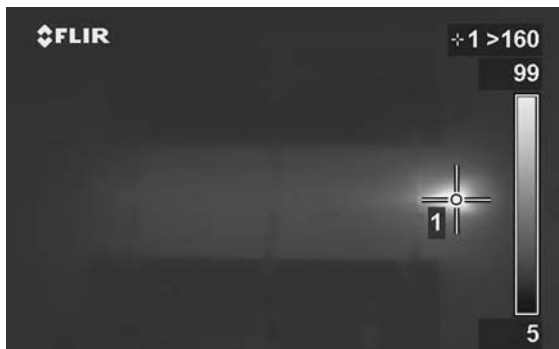
Figure 7a: SLIVER cells without reverse breakdown protection (RBP) breakdown at one end and heat beyond 160°C at currents around 3x Isc (100mA)
