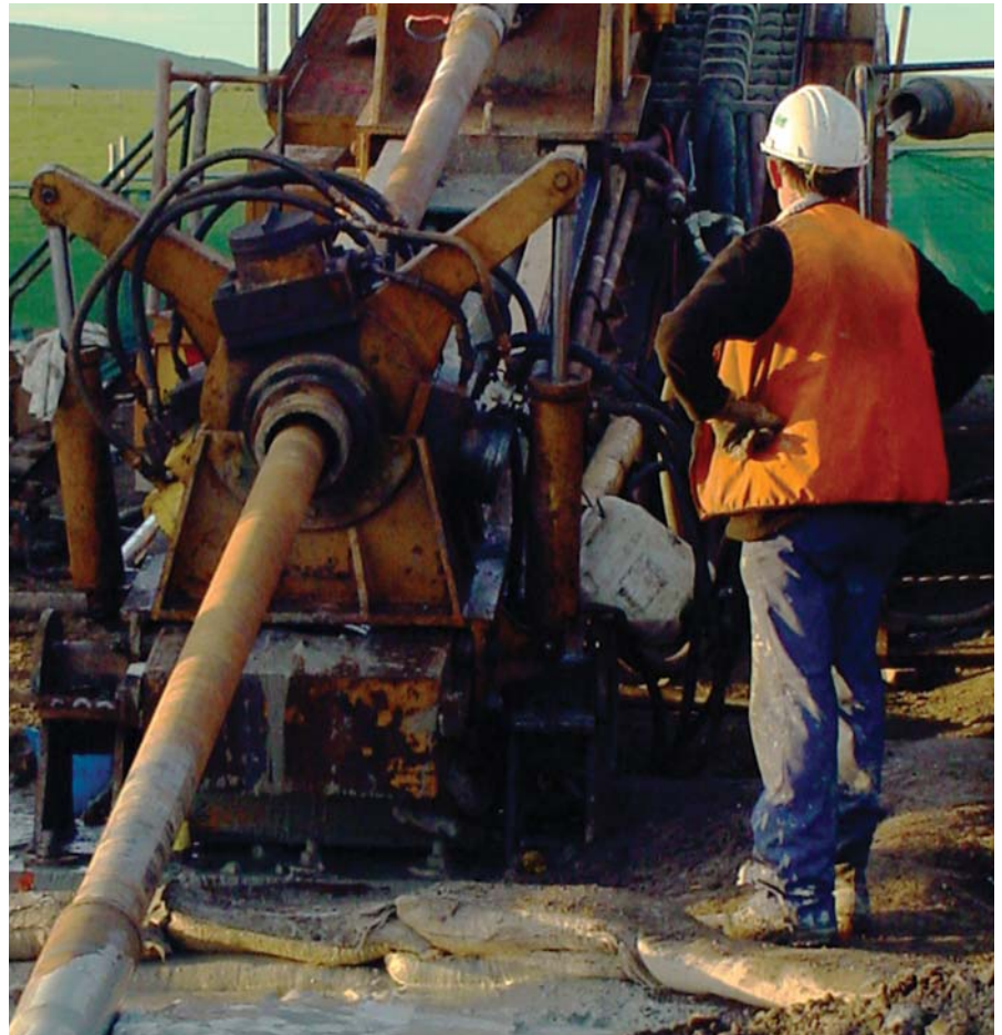
Figure 7: This machine is a type of drill rig that is proposed to be used in a drilling program that will avoid environmental disturbances near the shoreline.
